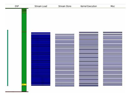
The longer green bar represents the entire DSP MIPS execution time of the program. The smaller bar to its left is the <code>sad\_16x16</code> pipeline timer. The almost solid bar in the Stream Load column shows that load bandwidth is the limiting performance factor for this pipeline. The spaces between the horizontal bars in the Stream Store and Kernel Execution columns represent time that the stream controller store unit or the DPU is idle while waiting for a dependency to be fulfilled.
