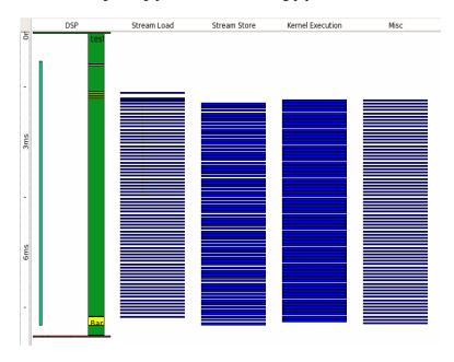
The longer green bar represents the DSP MIPS execution of the entire program, while the smaller bar to its left is the **error\_disperse** pipeline timer. The almost solid bar in the Kernel Execution column shows that the DPU is the limiting performance factor for this pipeline. A magnified view from the middle of the pipeline shows more detail:
